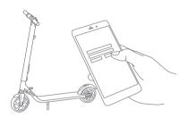
Power on the KickScooter. A blinking Bluetooth icon indicates the KickScooter is waiting for a connection.
