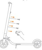
3. Install the battery pack onto the support bracket and tighten the screws securely.
