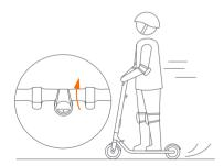
4. Slow down by releasing the throttle;stir the brake handle thumb shifter quickly and stamp the fender with foot at the same time to trigger mechanical braking in order to make a sharp brake.
